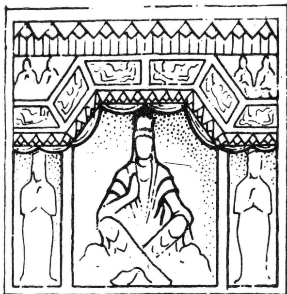
五面券 FIVE-SIDED ARCH WITH 券面作斜方格 TRAPEZOIDAL PANED EXTRADOS
