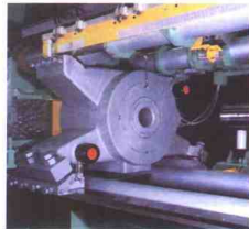
四点定位之最大铁箱 Four-Point Locating Of Container
