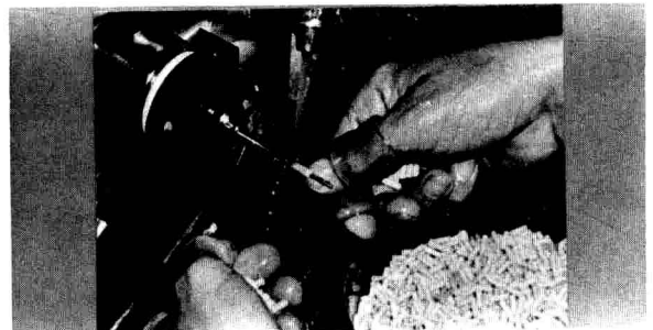
Honing of alumina tube blanks
