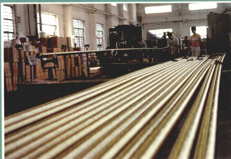
燕達廠鋼絲纏繞高壓膠管生產線 Production line of high-tension rubber hoses with steel wire of Yanda Rubber & Plastic Products Factory
