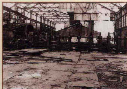
中国电力制钢厂建成的横列式小轧机 Mini rolling mill laid out in horizon built by China Electrical Steel Works
