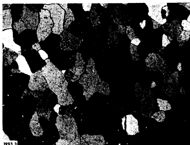
Figure 3. Microstructure of a Zircaloy-2 plate fabricated by developed schedule, showing reduced preferred orientation, absence of intermetallic stringers, but presence of small gas stringers: chemically polished, anodized; polarized light. \times 350
