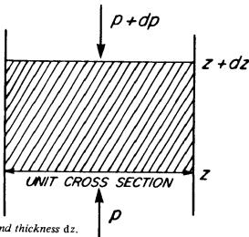
Fig. I-2. Layer of air column of unit cross section and thickness dz.
