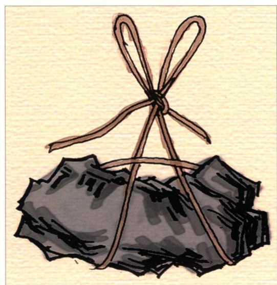
扣石绳结法 Method for Tying Ropes for Hanging Rocks
