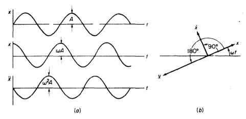
Figure 1.1-3. In harmonic motion, the velocity and acceleration lead the displacement by  $\pi/2$  and  $\pi$ .
