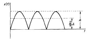
Figure 1.3-1. Average value of a rectified sine wave.
