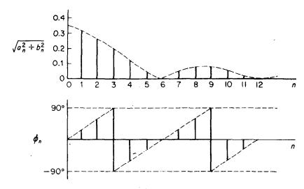
Figure 1.2-2. Fourier spectrum for pulses shown in Prob. 1-16, k = 1/3.
