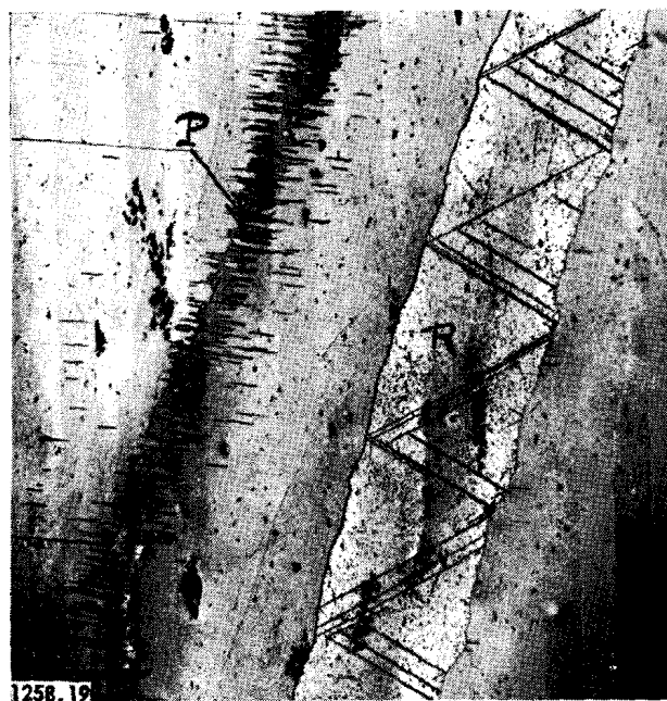
Figure 19. The same imperfect crystal, as hardened by strain, gives after annealing a recrystallization crystal, R, which develops along the distortion strips, and an imperfect serrated-contour crystal, P, at the level of the short twin crystals formed on a subgrain of the original crystal ( \times 40 )
