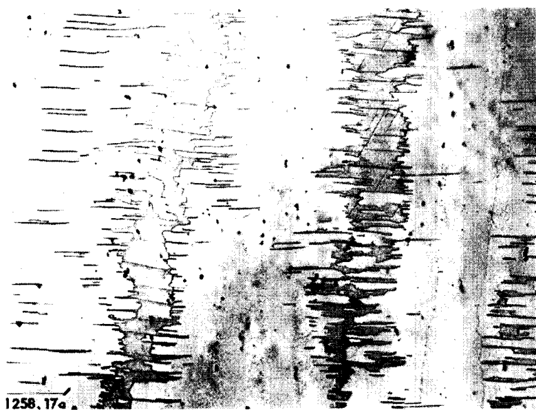
Figure 17a. After annealing at 640°C there is a recrystallization process along the same subgrains ( \times 150 )
