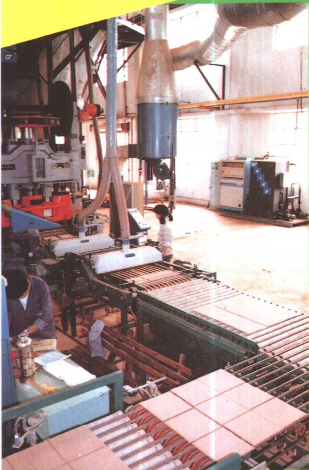
利華裝飾磚廠從意大利引進的牆地磚生產綫 The inputed automatic productive line for wall-floor tiles of Lihua Decoration Wall-floor Tiles Factory.
