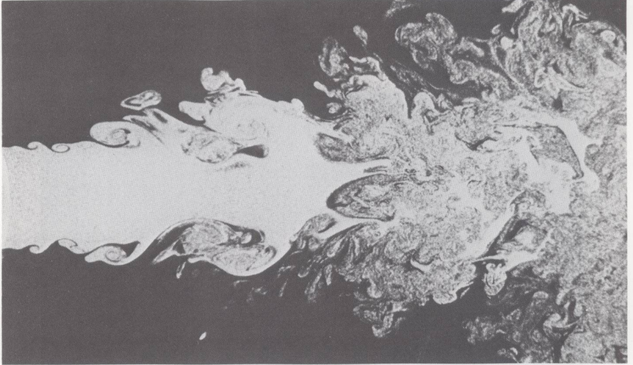
Figure I-2: turbulent jet ( picture by J.L. Balint, M. Ayrault and J.P. Schon, Ecole Centrale de Lyon; from [1], courtesy J.P. Schon and “La Recherche” )
