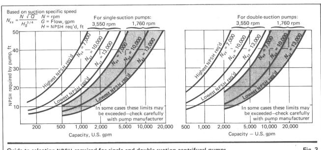
Guide to selecting NPSH required for single-and double-suction centrifugal pumps
