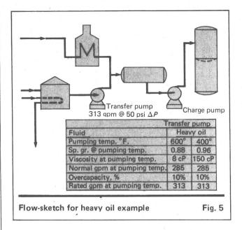
high (500 psi or above), reciprocating pumps probably represent the best choice. Manufacturers' data or Hydraulic Institute methods will help determine how much to derate the capacity of a reciprocating pump for viscous liquids.
