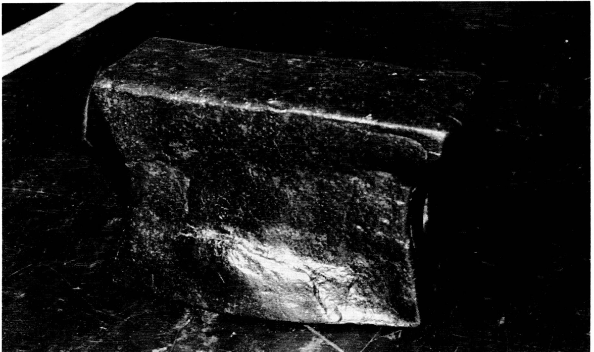
Fig.1-1. This medieval anvil without horn or holes was probably used by an armourer.
