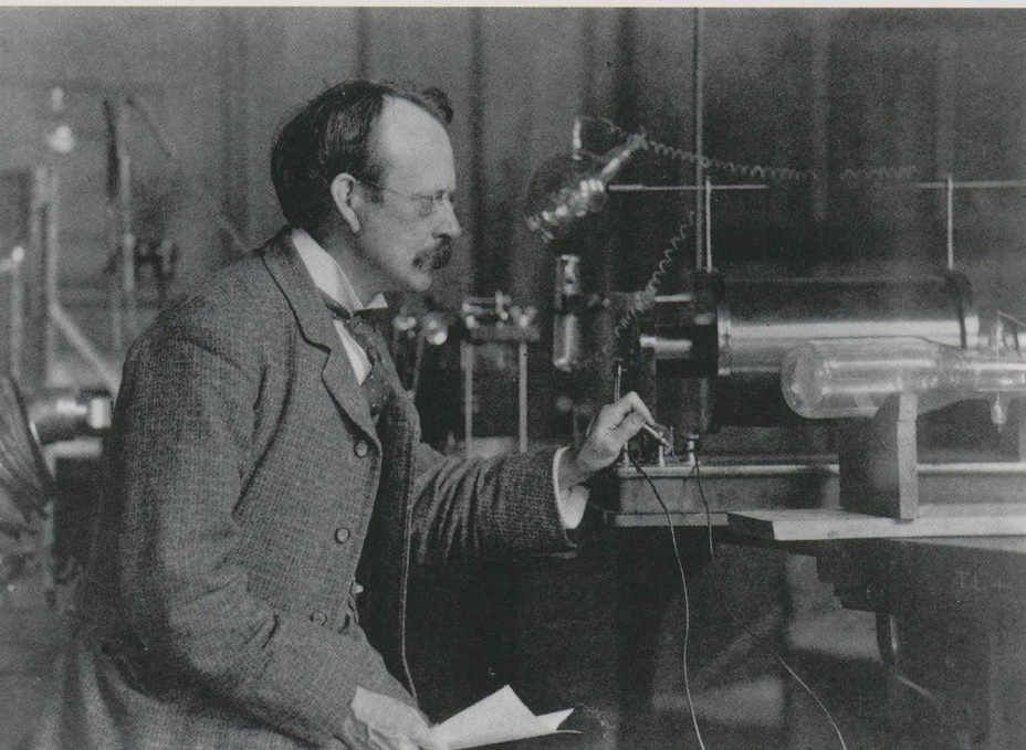
British physicist J. J. Thomson ushered in a new era of subatomic physics by discovering the electron in 1897. Here he is shown in the 1890s with the apparatus he used to determine the ratio of the electron's electrical charge to its mass.
