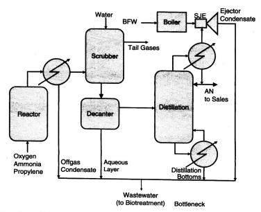
FIGURE 1-1a PROCESS FOR AN MANUFACTURE (EL-HALWAGI 1997)
