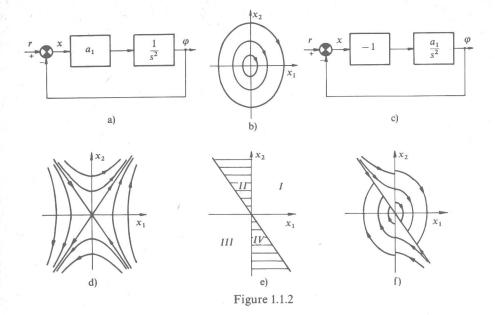
(Figure 1.1.2c), the system is aperiodically unstable and is described by the equations
