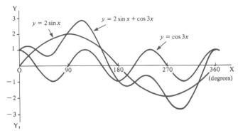
Many technological situations give rise to compound periodic waveforms and, in order to study one such output, it is convenient to analyse it into a number of component sine and cosine constituents. Such a process is therefore the reverse of that employed in the three examples worked above. Just how this analysis is achieved is explained in detail in a later chapter.
