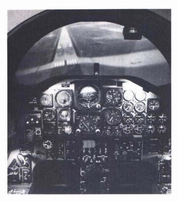
At Williams Air Force Base, near Phoenix, Arizona, pilots train in this cockpit which uses simulation technology to recreate flight conditions. The scene displayed on the screen in front of the pilot gives the illusion of flight.
