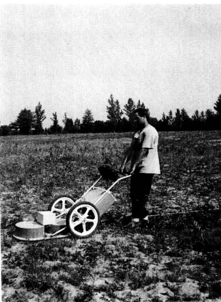
A georadar unit is walked across the site. Subsurface anomalies such as walls and fireplaces may appear in the images from the instrument.
