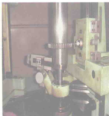
40. 用渐开线检查仪测量齿廓总误差 F_\alpha
