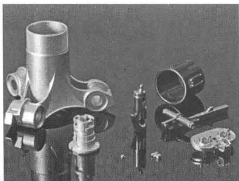
图1-1 精选的0.028~260g的MIM零件
