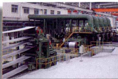
自主研发的全新八辊五机架冷连轧机组 Independent researched and developed latest 8-rollers 5-stands cold mill
