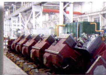
自主研发的保证轧制速度105m/s的新型顶交高速线材精轧机组 Independent researched and developed new-type top cross high-speed wire and rod mill which can guarantee the mill speed of 105 m/s
