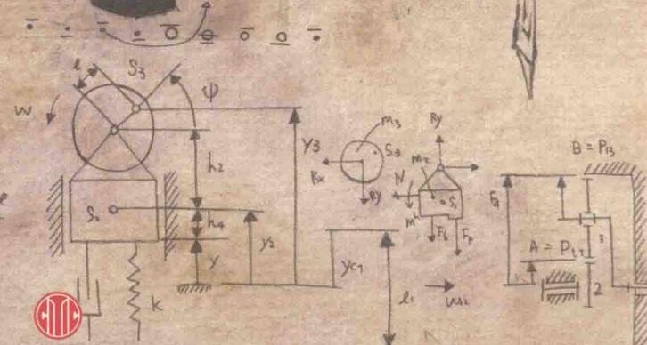
$$M_2 \ddot{y}_2 = -F_b - F_p + Ry \quad M_3 \ddot{y}_3 = -Ry \quad W_{14} = \frac{r_2}{k_1 + r_2} W_{12}$$
