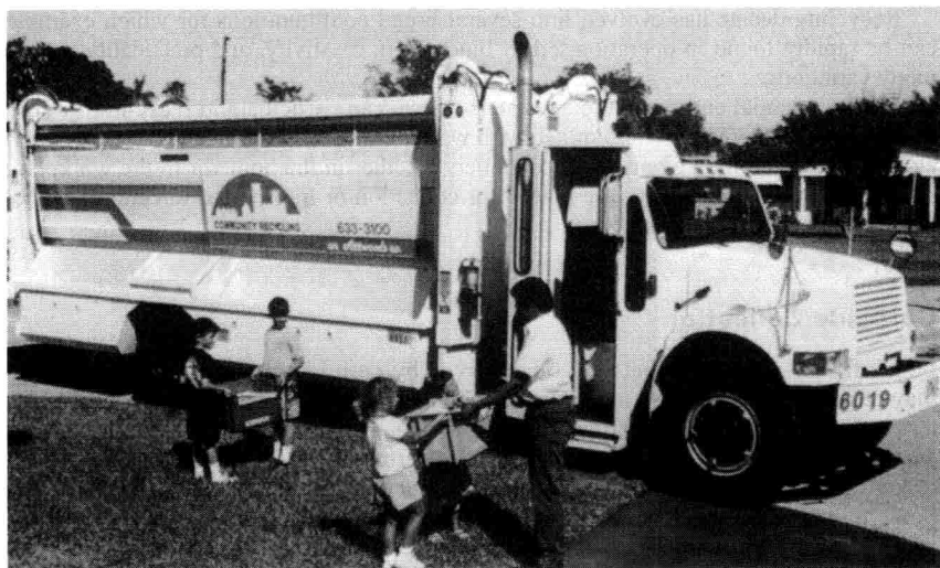
FIGURE 1.4 Specialized curbside recycling materials: collection truck with compartments, dual sides, and hydraulic top loading.
