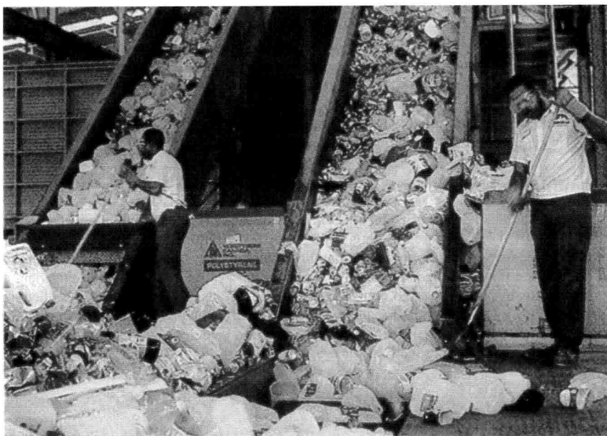
FIGURE 1.5 Materials recovery facility (MFR) infeed conveyors for commingled materials at Community Recycling, an Attwoods Company in Dade County, Florida, that serves over 265,000 homes.
