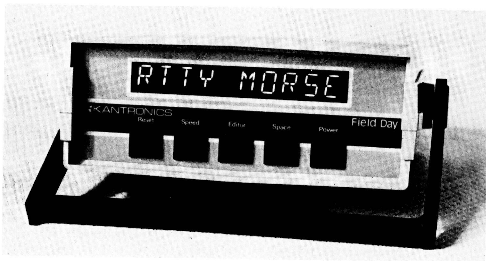
Figure 1-4. Kantronics Field Day 2 Morse and RTTY Reader (a microcomputer-based product). (Courtesy Kantronics.)
