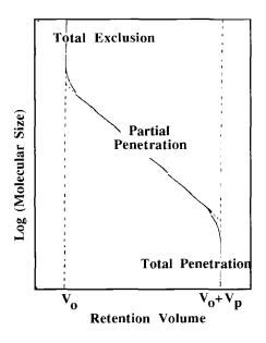
The slope of the line between the limits of total exclusion and total penetration controls the component capacity and the resolution possible.
