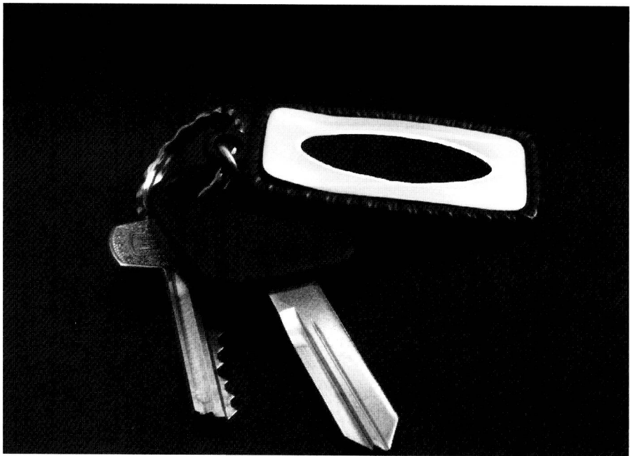
Figure 1 The Immobilizer is built into the housing of the auto key. (Image reprinted courtesy of Texas Instruments Inc.)
