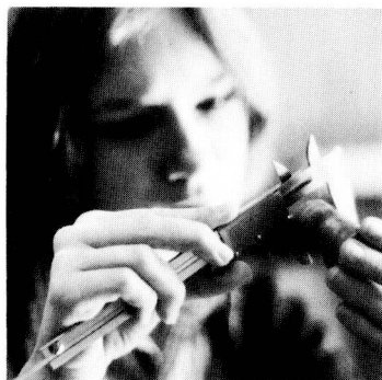
FIGURE 1-7 Common scientific measuring instruments. (a) A vernier caliper, designed to measure inside or outside dimensions to 0.1 mm. (b) A micrometer caliper, which measures outside dimensions to 0.01 mm.
