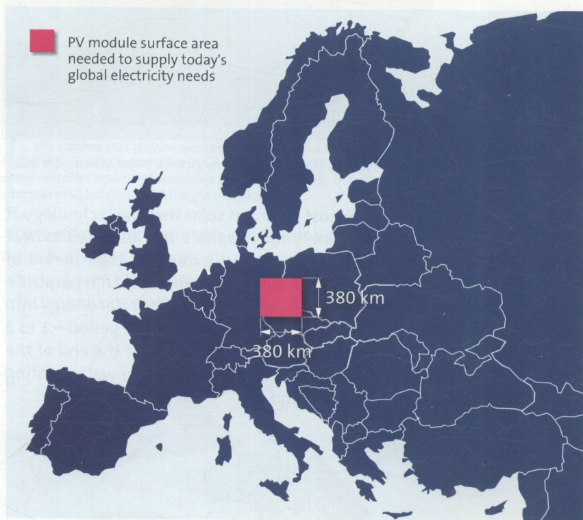
Figure 1.10: A PV array covering 1.5% of the European land mass would be enough to supply current global energy demand (based on global electricity requirement of 17,300 TWh – tera-watthours, one trillion watthours (2005) and a 145,000 km 2 PV array in central Europe with an efficiency of 12% generating 120 kWh/m 2 /year)
