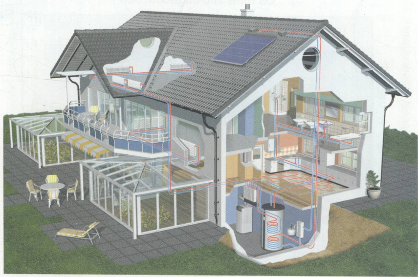
Figure 1.6: Design for a house in Central Europe with several passive solar features, such as conservatories and small windows on the north side. The central heating system is solar thermal assisted (Source: http://www.elco.net )
