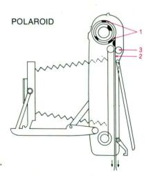
The 'Polaroid-Land' process, which produces positive pictures in a few seconds, incorporates a self-developing gelatine pellet (1), which is spread over the film by the rollers (3), and makes the positive print (2) by contact with the negative image. In this way the conventional developing and printing processes are eliminated.
