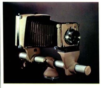
Left: A monorail camera (Linhaf) which can correct for distorted perspective. By means of swings and tilts about the lens and film planes, effects such as the converging of verticals when looking at a building from above or below can be controlled or eliminated. Below left: Photograph taken without corrections to alter 'false' perspective. Right: Correction by altering the lens axis. The diagram shows the tilt used for such a photograph.
