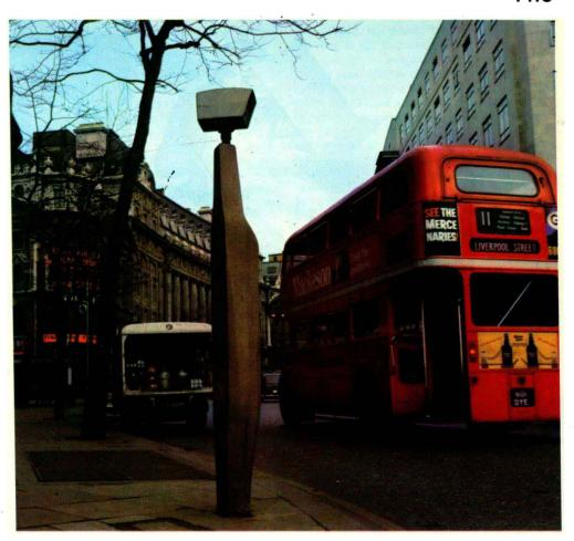
A London bus passes a photoelectric scanner. This directs a beam of light on to individually coded light-reflection equipment on the side of the bus, so that its progress through London's crowded streets can be traced by a central control room and, if necessary, some action taken.
