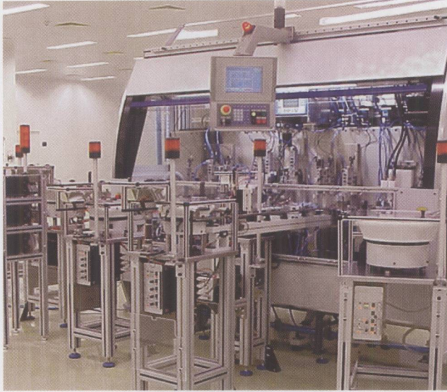
FIGURE 9.14 (d) Robotic system for mounting and assembling Respimat.
