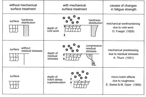
Fig. 1.1: Approaches for the explanation of changes in fatigue behaviour due to mechanical surface treatments
