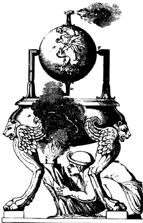
Fig.1: "Turning sphere", quoted by Hero of Alexandria, 120 b.c.
