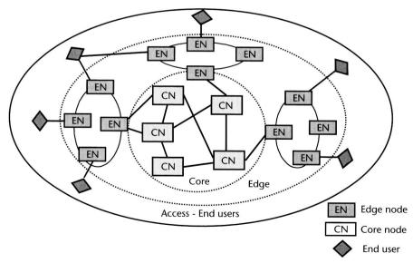
Figure 1.1 Optical networking structure.
