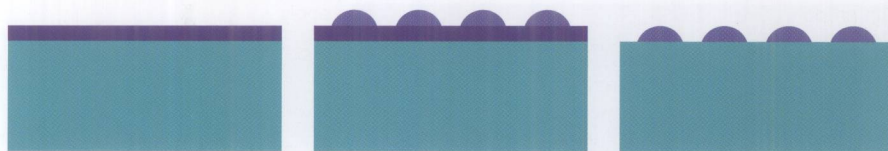
Plate 7 Schematic of three thin film growth modes. Left: Frank–van der Merwe or planar layer-by-layer growth. Center: Stransk–Krastanow or island growth on a wetting layer. Right: Volmer–Weber or island growth with no wetting of the substrate.
