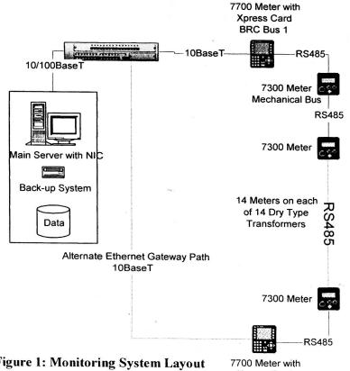
Figure 1: Monitoring System Layout
