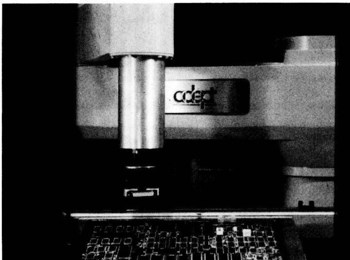
Figure 1.4 Adept vision guided robot shown stuffing components into printed circuit board.
