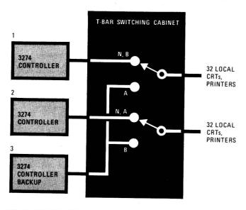
channel with the standby 3274 from the 2914 panel. As shown in Figure 1, the T-Bar cabinet switching control unit, reacting to a failed IBM 3274 control unit, would switch all 32 devices from the faulty 3274 to the standby unit. An on-line command restores the 32 devices. Total downtime lasts less than 1 minute.
