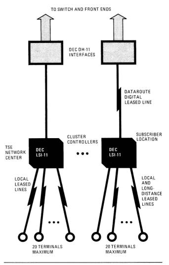
digital leased lines, which are substantially less-expensive than standard voice-grade lines. About half of the 1,350 Autodat terminals are linked to the network center over these facilities.
