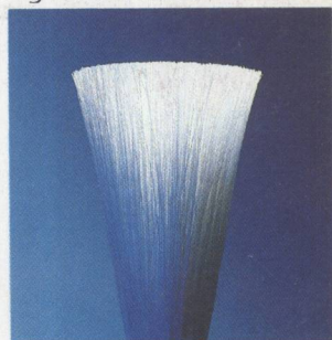
Microporous hollow fibers used in Capiox II
