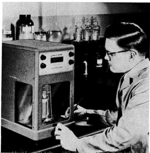
Fig. 1-7. Modern analytical balances are used to weigh accurately to 0.0001 gram.
