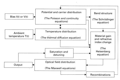
Fig. 1.1. The physical processes and their linkages in the operation of optoelectronic devices. Noted in brackets are the first principle equations that govern these processes.
