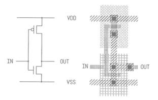
VDD is connected to the metal wire on top, VSS is connected to the wire on the bottom. The input signal enters in polysilicon on the left and forms the gate of two transistors, an N-transistor on the bottom and a P-transistor on the top. The bottom N-transistor turns on when IN is high, connecting OUT to VSS. The top P-transistor turns on when IN is low, connecting OUT to VDD.
