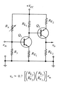
Figure 1.2 Discrete form of direct-coupled amplifier: it requires calculation of proper values of at least six resistors to accomplish desired gain; compare this to a simple ratio of two resistors for the OP AMP in Fig. 1.1.
