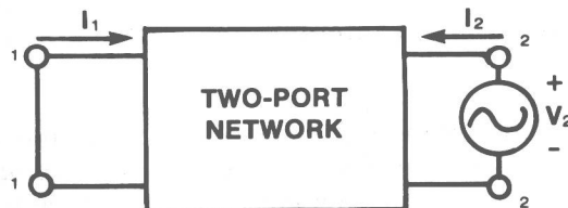
Arrangement for determining Y_{22} and Y_{12}
