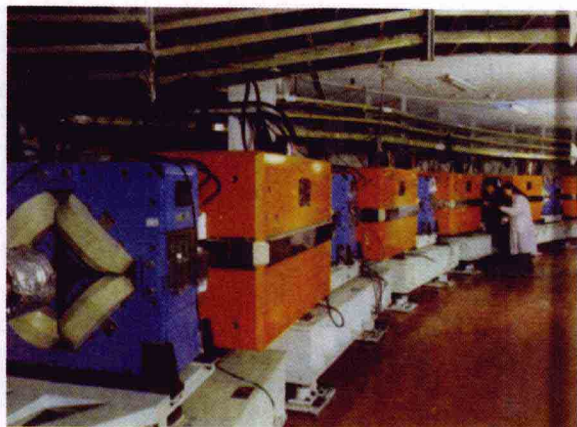
Fig. 0-6 The positive and negative electron colliding machine in Beijing, China, used for exploring the motion laws of microcosmic particles. (The figure shows the store ring of the machine.)
