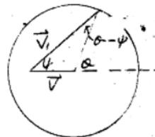
$$\text{但 } \frac{\sin(\alpha-\psi)}{\sin\alpha} = \frac{V}{V_1} = \frac{m_1}{m_1+m_2} \quad \frac{U_1}{V_1}$$
