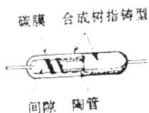
铸型皮膜电阻 (c) 碳膜电阻
