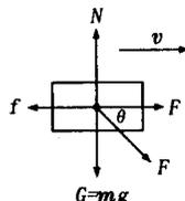
$$\left. \begin{aligned} F + F\cos\theta - f &= 0 \\ N - mg - F\sin\theta &= 0 \\ f &= \mu N \end{aligned} \right\} \quad (3)$$
