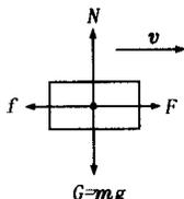
$$\left. \begin{aligned} F-f &= 0 \\ N-mg &= 0 \\ f &= \mu N \end{aligned} \right\} \quad (1)$$
