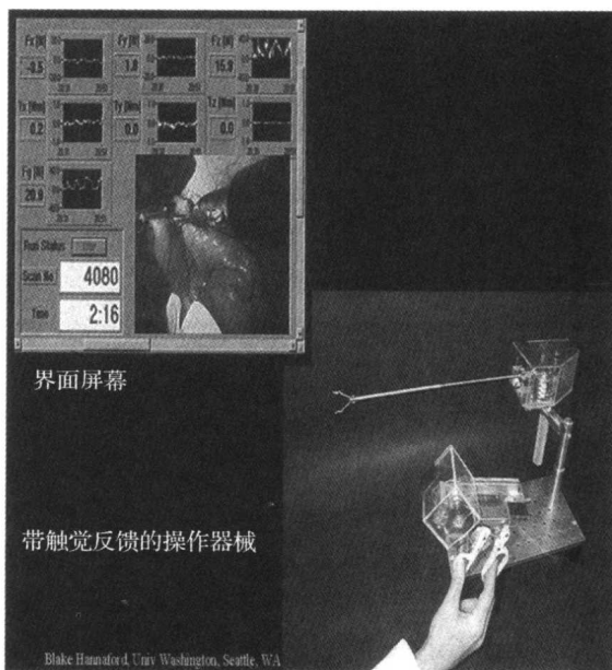
图1-3 改进后的具有感觉功能的腹腔镜器械,在监视器上展示手术操作(Courtesy of Blake Hanaford, PhD, Department of Mechanical Engineering, University of Washington, Seattle, Wash.)
